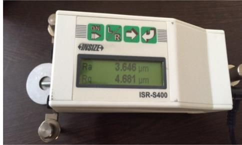
Fig. 4. Surface roughness tester.
